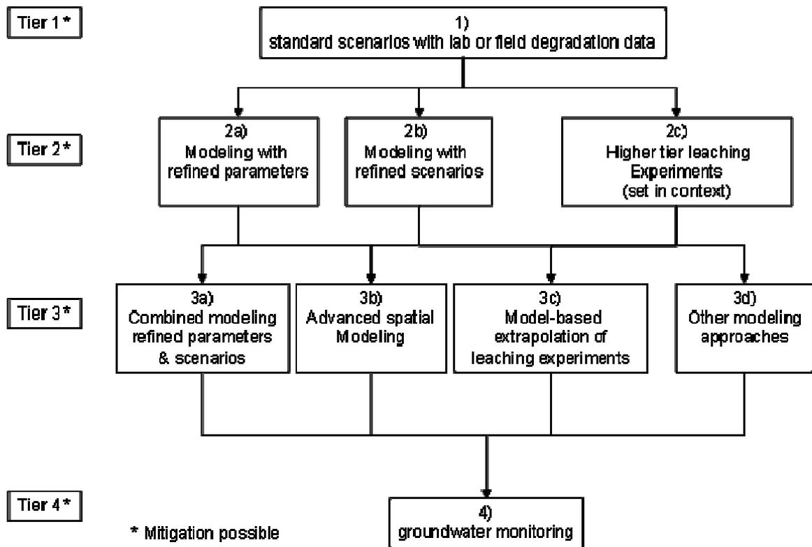
**Figure 2 : FOCUS proposal for generic tiered assessment scheme for ground water**
